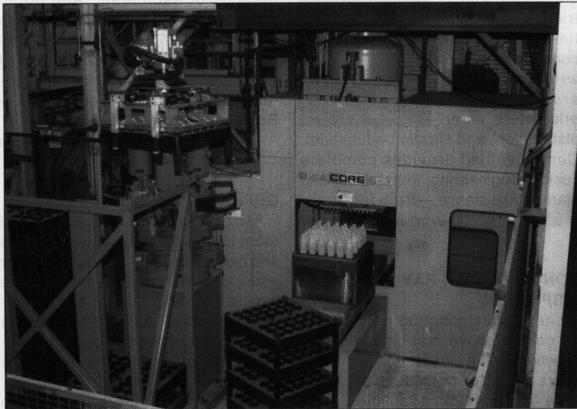
The Core 300 features a core removal system that is used with an ABB robot for quick and precise core removal and handling.
